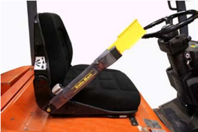
The Safe-Belt is designed to irritate the operator until the seatbelt is fastened. The bright yellow end is easily seen to ensure the operator is wearing it.
